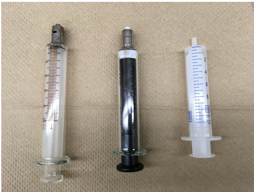
10 mL syringes. From left to right: glass-barrel, gas-tight, and disposable. Note the metal Luer lock fittings on the glass-barrel and gas-tight syringes.
