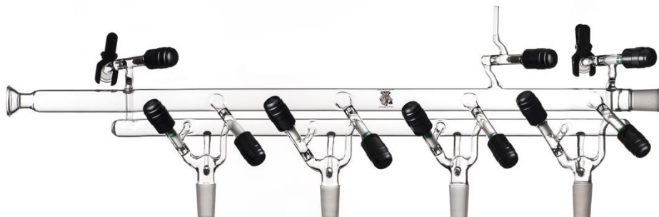
The typical UW Schlenk line. The upper line connects to a vacuum pump via a solvent trap. The lower line is filled with N 2 through one of the top ports. The four lower ports allow for N 2 or vacuum to be applied to the connected glassware.
