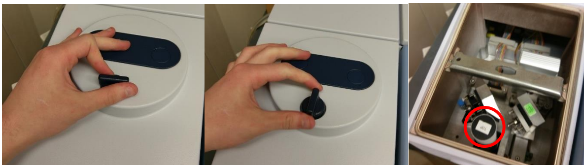
Lid to first sieve compartment. Left: lid in closed position, middle: lid in open position, right opened lid compartment. Circled in red is the cylinder containing the sieves.
